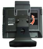
Remove the detachable base by pressing upward to remove the cover, then unscrewing the four screws attaching the base to the display.
